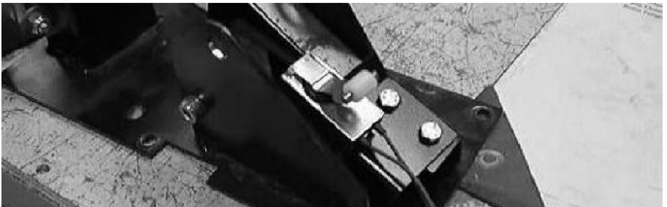
FIG. 2 - MOUNT ROLLER SWITCH TO MOUNTING BRACKET
