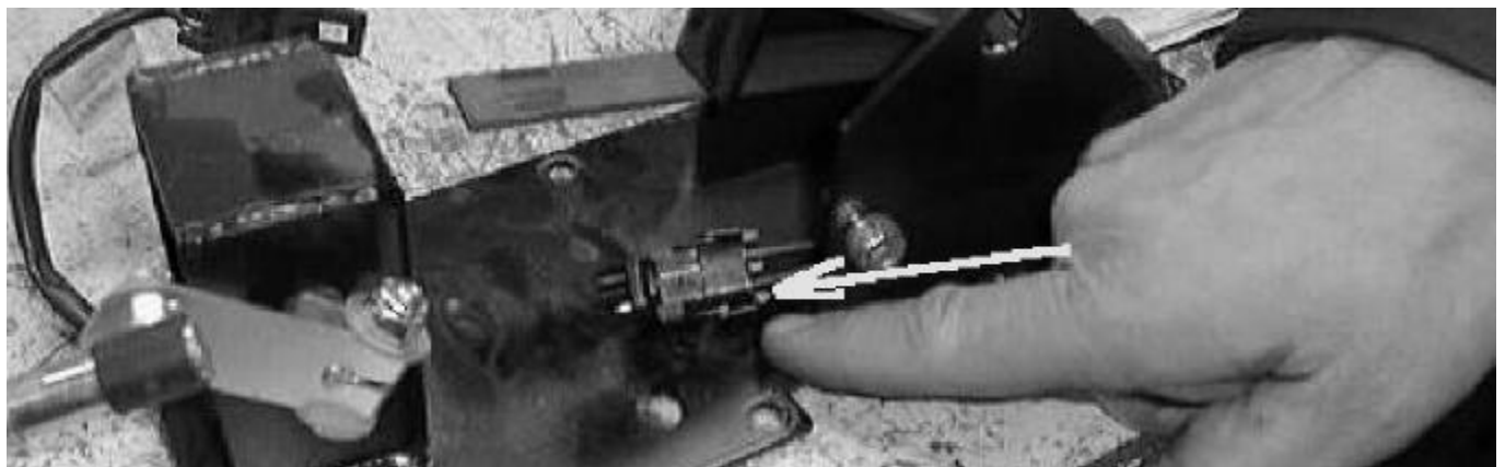
FIG. 3 - MOUNT SWITCH ASSEMBLY TO PROPELLING PEDAL
